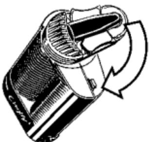
Screw the Cooling Unit onto the Vaporizer by turning 90° clockwise.
