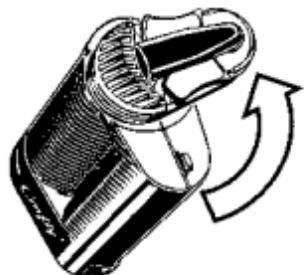
Unscrew the Cooling Unit from the Vaporizer by turning it 90° counter-clockwise.
