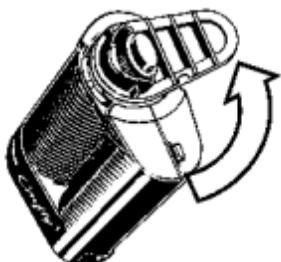
Unscrew the Cooling Unit base from the Vaporizer by turning it 90° counterclockwise.
