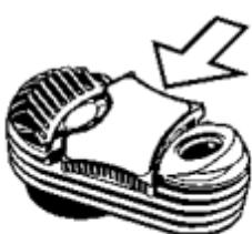
First press the cap lock on one side and pull it up on the opposite side.
