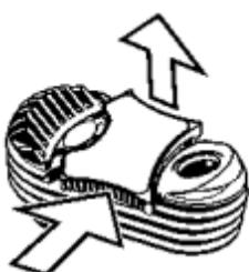
When cleaning the Cooling Unit Cap in isopropyl alcohol, remove the cap lock by pulling it up on one side.
