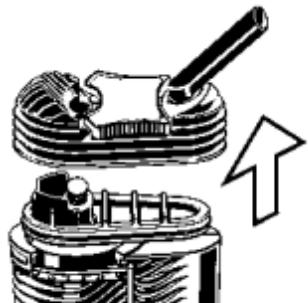
Pull the Cooling Unit Cap off the Vaporizer.
