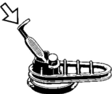
Press the Screen with the Filling Chamber Tool from the top to the bottom out of the Cooling Unit base.
