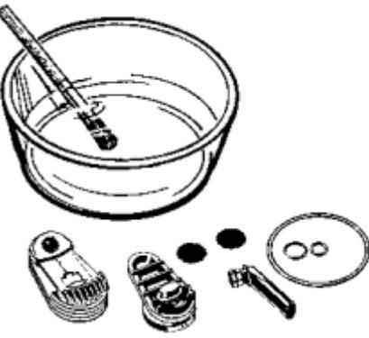
Place all parts of the Cooling Unit in warm rinsing water.
