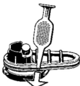
Lever out the large Base Seal Ring with Filling Chamber Tool at the recess in the groove. Remove the small Base Seal Ring.
